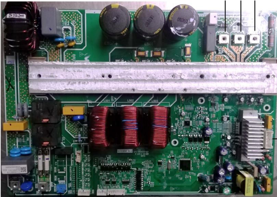
Figure 4-1.4: 36/42/48/56 model outdoor unit communication switchboard
